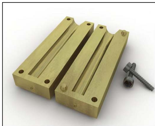
Fig. 1. Metal molds used for starch consolidation casting.
